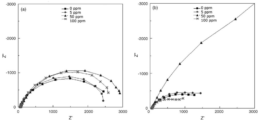
Fig. 6. Nyquist diagrams with amine type inhibitor concentration of 0, 5, 50 and 100 ppm corresponding to electrochemical test in (a) static system and (b) dynamic system (1500 rpm).
