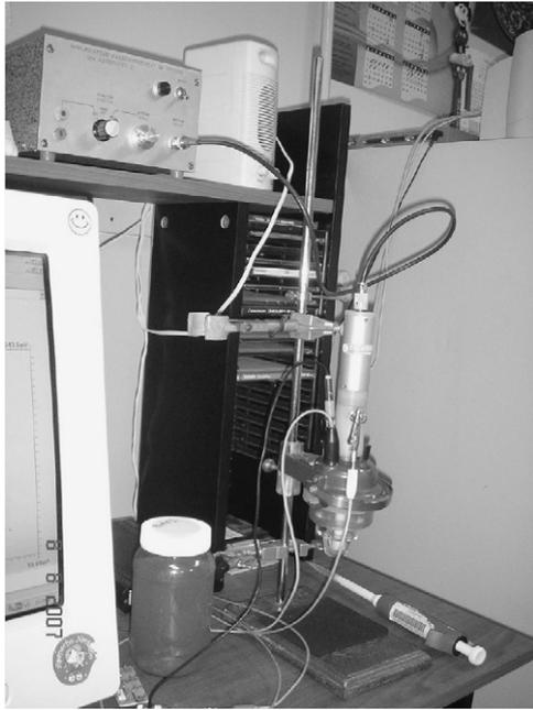
Fig. 4. EIS cell experiment with a rotational speed of 1500 rpm.
