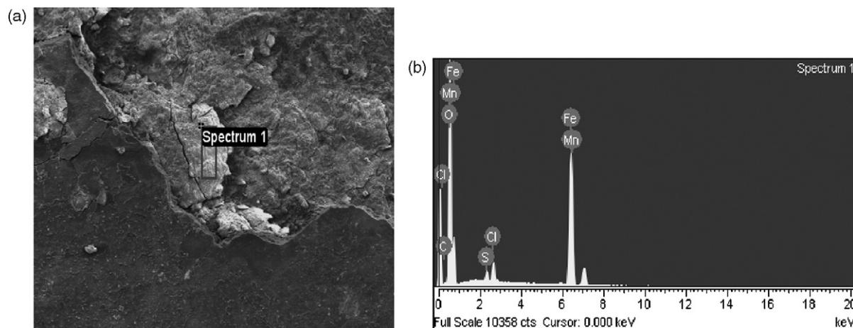
**Fig. 7.** (a) SEM micrograph corresponding to sample tested in dynamic extended system test, 100 ppm amine concentration and (b) EDS analysis showing presence of Cl and S.
