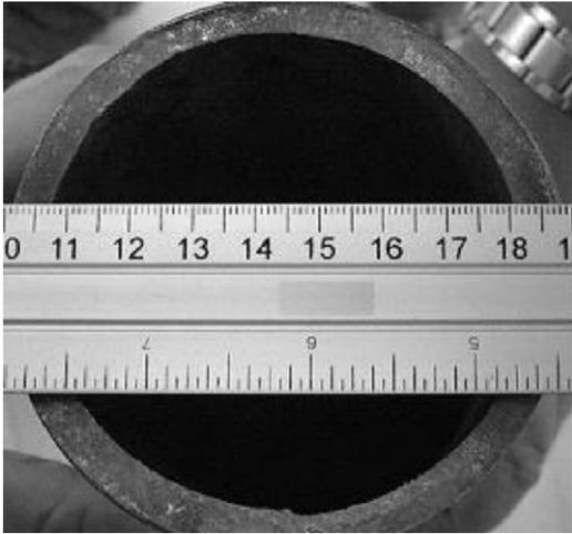
Fig. 1. Natural gas pipe section of 101.6 mm diameter of an API X52 steel grade.
