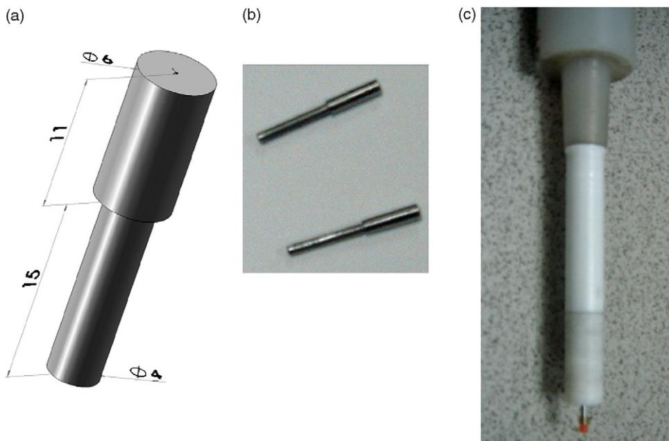
Fig. 2. (a) Schematic representation of the sample (mm) used in electrochemical test, (b) final sample machined and (c) mounted sample with an exposed area of 18 mm<sup>2</sup>.
