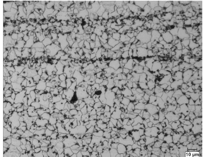
Fig. 3. Microstructure of the pipe section showing a typical microstructure of an API X52 steel grade containing pearlite bands phase in a ferrite matrix, 400 $\times$ .
