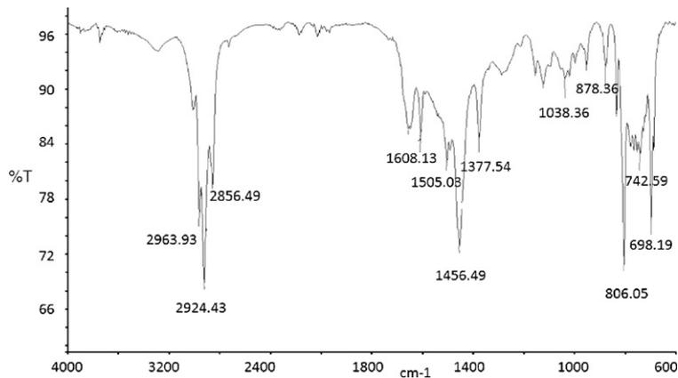
Fig. 5. Infrared spectroscopy spectrogram of the amine type inhibitor.
