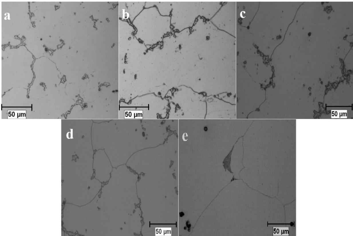
FIGURE 2. SEM images showing the progressive carbides dissolution according to heat treatment time in CT; carbides change from lamellar to a round-like morphology before being dissolved. a) Sample II. b) Sample III. c) Sample IV. d) Sample V. e) Sample VI.
