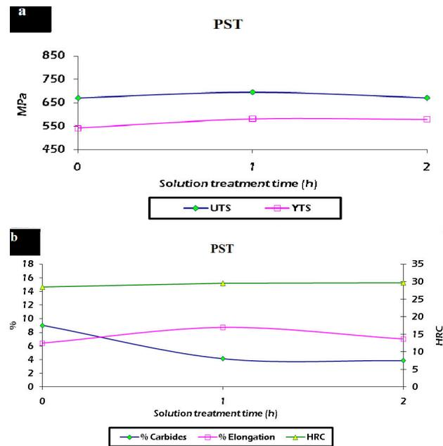
FIGURE 6. Mechanical properties behavior and relation between carbides percentage, elongation and hardness in function of the heat treatment applied for PST. a) YTS and UTS. b) Carbides content, elongation and HRC.
