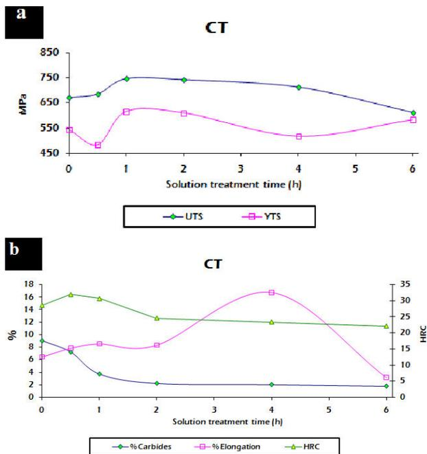
FIGURE 5. Mechanical properties behavior and relation between carbides percentage, elongation and hardness in function of the heat treatment applied for CT. a) YTS and UTS. b) Carbides content, elongation and HRC.
