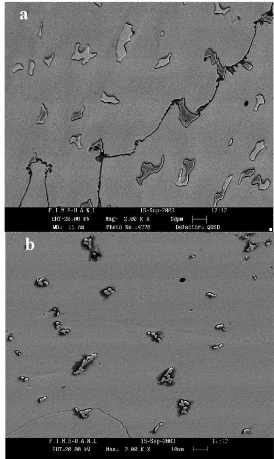
FIGURE 4. SEM images showing the carbides morphological evolution on PST. a) As cast lamellar carbide. b) Round-like carbides after PST.
