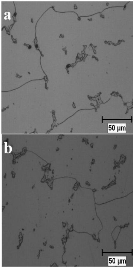
FIGURE 3. Optical micrographs showing the carbide dissolution according to time of PST. Carbides did not dissolve completely; only change its morphology from lamellar to globular. a) Sample VII. b) Sample VIII.
